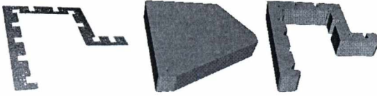
Figure 4: Concave problem - points of a concave roof segment (left) - triangulation on the whole convex hull (middle) - triangle mesh generated by our method (right)
