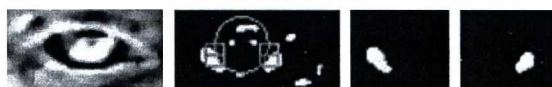
Figure 2: Homogenous sclera, candidate sclera regions and rectangular search windows, selected left and right side sclera segments (left to right)
