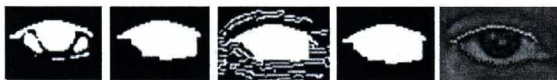
Figure 3: Eye mask, filled eye mask, vertical edge based extension, final eye mask, upper and lower eyelid contours (left to right)
