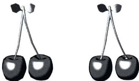
Figure 3: Silhouette detection using the facing ratio (the dot product of the view vector and the shaded normal) of shaded points. The cherry model on the right is highly tessellated which results in higher quality contours.
