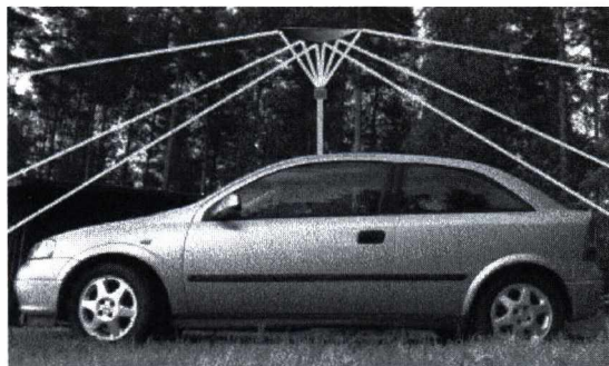
Figure 13: Sketch of a catadioptric system – comprising an upward-looking camera and a rotational symmetrical non-planar mirror with an apex – mounted on a host vehicle. The camera and the mirror are rigidly mounted on a rod.
