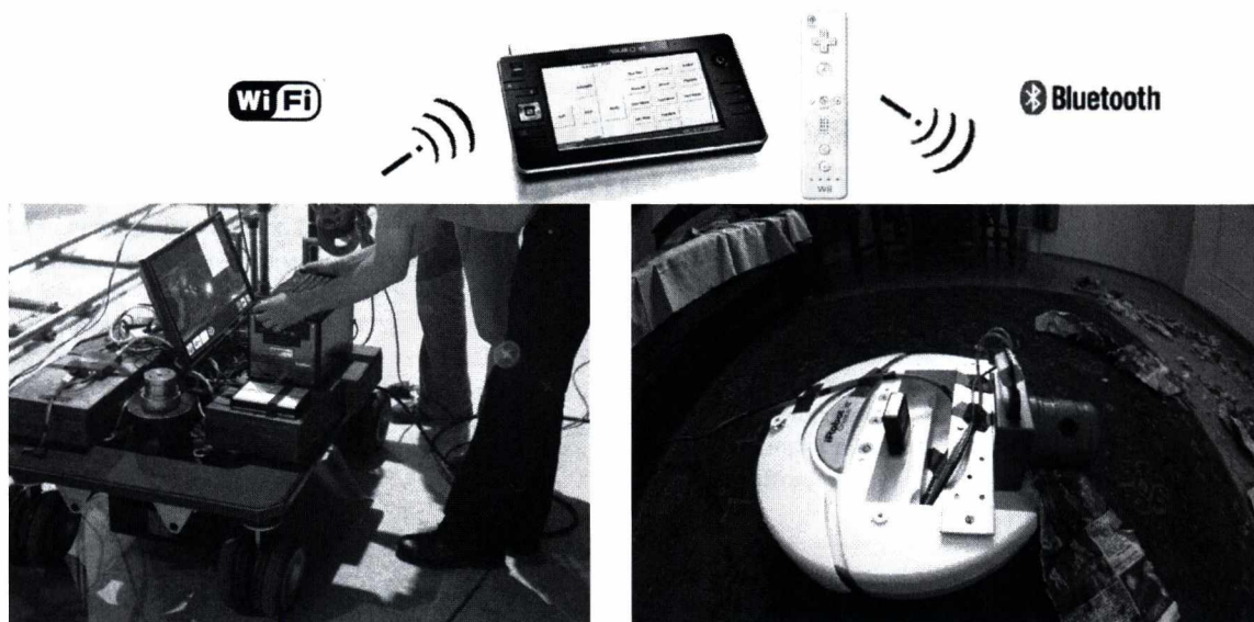
Figure 7: Remote controlled robot camera used to record the panoramic videos for the Metamorphosis (see text for details).
