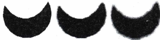
Figure 8: Shadow mask before blur, after horizontal blur and after horizontal and vertical blur.
