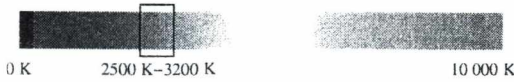
Figure 7: Black-body radiator colors from 0K^{\circ} to 10000K^{\circ} . Our demo used temperature values from 2500K^{\circ} to 3200K^{\circ} .
