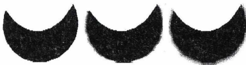
Figure 9: Shadow mask before blur, after horizontal blur and after horizontal and vertical blur. Note that shadow mask is not blurred at the upper edge, because here the occluder meets the shadow receiver.
