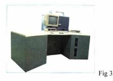
The development of the first Bulgarian mini-computer started in 1974, using as a prototype PDP8L of the company DEC. The mini-computer was known as IZOT 310 and its word was 8 bits and time for execution of the instruction-  $2-12 \mu$ sec, main memory – 64 KB and UNIBUS interface.
