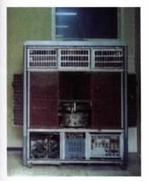
Fig. 1 – CRC 102-A. (1954) Drum memory is placed in central position. (Preserved at the Polytechnic of Milan)
