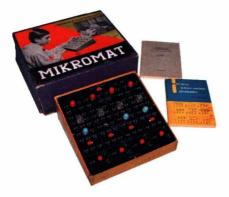
His student, Ferenc Woynarovich made the Mikromat cybernetic building kit. To introduce the basic principles of computer science, the computer model built of printed circuits contained four relays and eight bulbs and could be programmed by wires. With the help of this kit – for example with the construction of the game "The wolf, the goat, the cabbage and the farmer" one could easily learn the operating principles of the calculating and logical machines.
