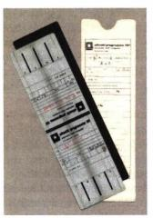
Fig. 13 – Floppy card for P 101; the black reverse is the magnetic-sensitive side. (7x25 cm)
