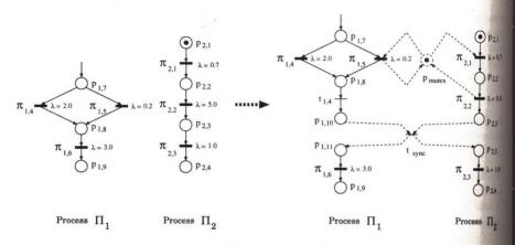
Figure 2: Modeling Process Interaction
